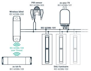
3 101 mode is enabled after a 101 power supply has been connected to the DALI terminal and the device has not been added to a 104 application controller.
