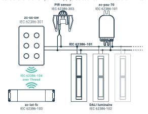
101 mode is enabled after a 101 power supply has been connected to the DALI terminal and the device has not been added to a 104 application controller.
